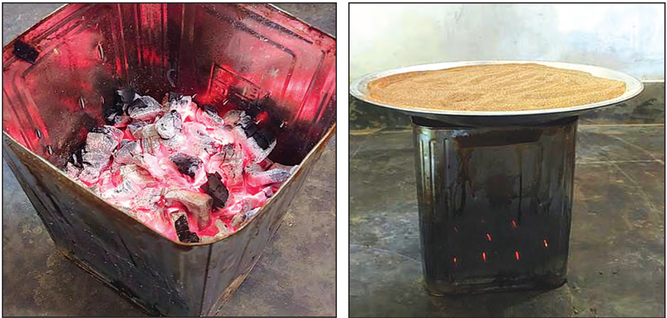
Fig 1: Low cost heating system (Using oil tin, charcoal, sand and iron pan)
