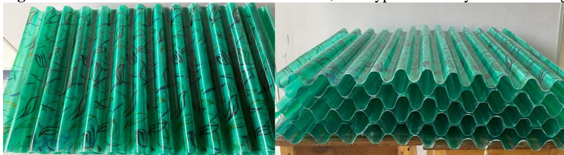
Figure: Layer-by-layer stacking of FRP sheets to arrive at the Honeycomb structure
